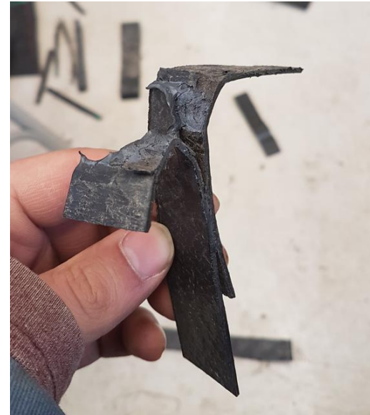
Failed Peel Tests
