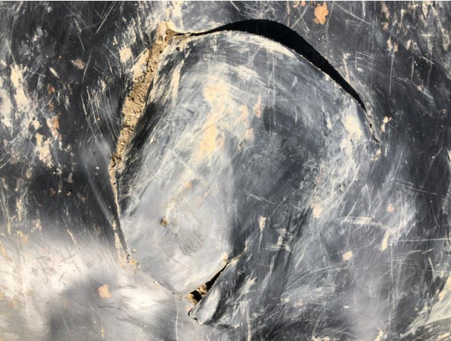
Damage from relocating waste
