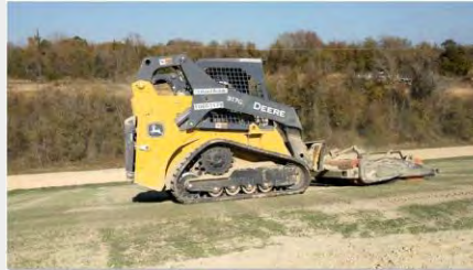
Sand Infill – Brushing and Grooming
