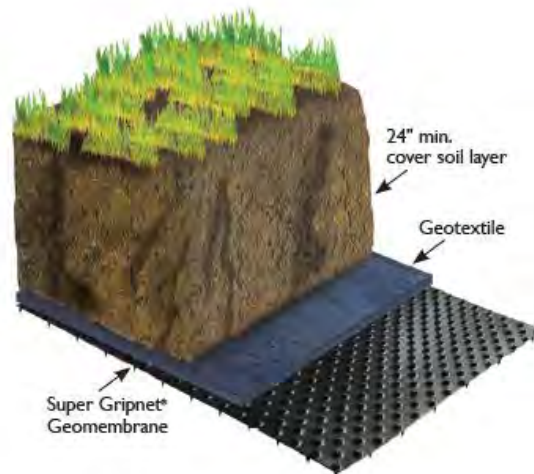
Integrated Drainage System (IDS)
