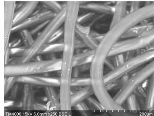
Nappe; 250X magnification (After aging).
