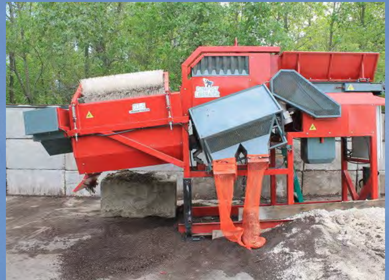
Contaminant Removal Unit at the Forks
