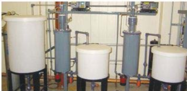
Completely automated BMP batch culture system, with unique individual flow meters
