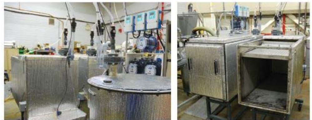
Dry Batch Digestion Pilot Plant (for non-flowing/stackable dry material)
