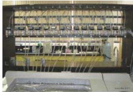
Completely automated BMP batch culture system, with unique individual flow meters
